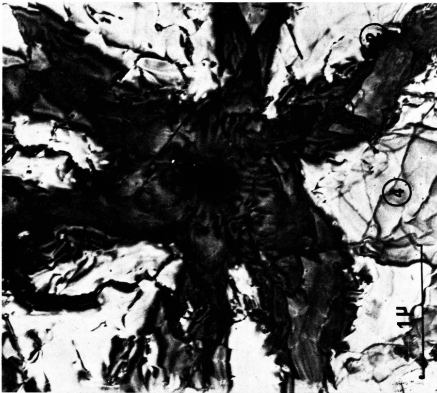
Fig. 3. Extinction contours near the [111] direction in a specimen consisting of 1000 \text{ \AA} of Au plus 200 \text{ \AA} of Ag. The various orientations 1, 2, 3 and 4 referred to in the text are shown and the circles at these points denote the probe size used. In practice these where selected by reference to the diffraction pattern with the probe focussed.
